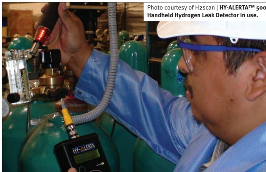
Photo courtesy of H2scan | HY-ALERTA™ 500 Handheld Hydrogen Leak Detector in use.
