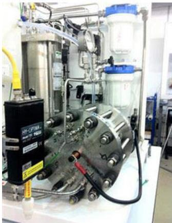
HFuel generates hydrogen by electrolysis, compresses it, stores it and dispenses the gas on demand at high pressure. The refueler is currently being used across the UK for the company's Hydrogen On Site Trials (HOST), which has already experienced broad support from organisations such as UK local authorities, DHL, UPS, the RAC, Tarmac, Amey, May Gurney, Scottish Water and Stansted Airport.
