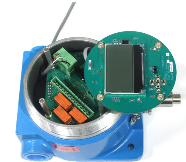
4. Pull any excess wire out of the enclosure.
