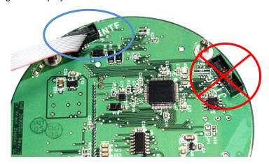
**Figure 2: Display Connections**
