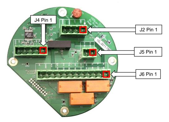
**Figure 3: Interface Board Showing Connectors**
