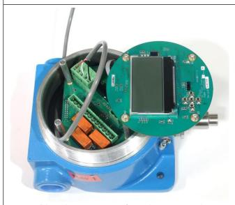
3. Plug the connector into the receptacle.
