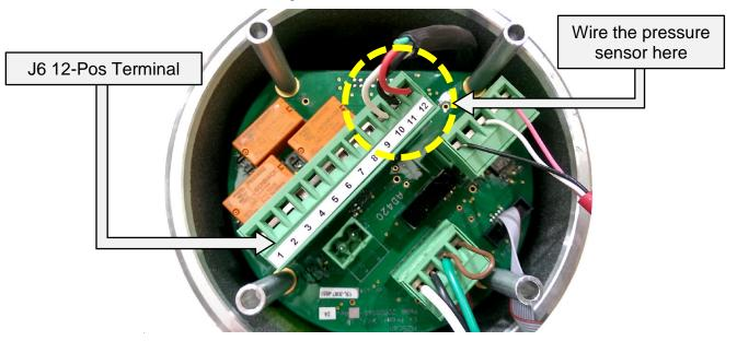
**Figure 5: Pressure Sensor Wiring**
