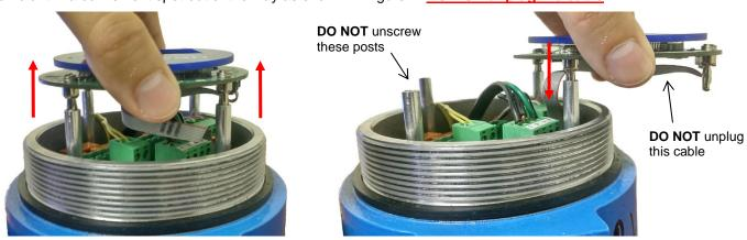
Figure 1: Removing the Display Board
