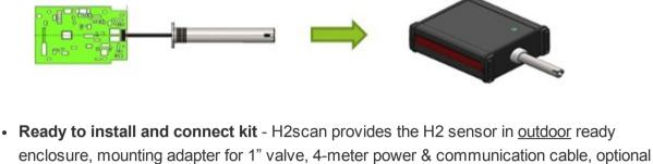
4-20mA analog output module, and 20 hours remote support to enable your team to integrate a solution onto your customer's new or existing transformers. (Designed for immediate field installation/integration with Modbus communications). Air Bleed Valve with DGA sampling port
