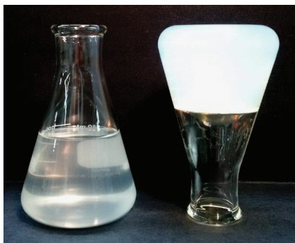
Fig. 3—10% active solution of PQ Corporation's EcoDrill S45 without setting agent (left) vs. 10% active solution of EcoDrill S45 with setting agent and set for 4 hours at room temperature (right).
