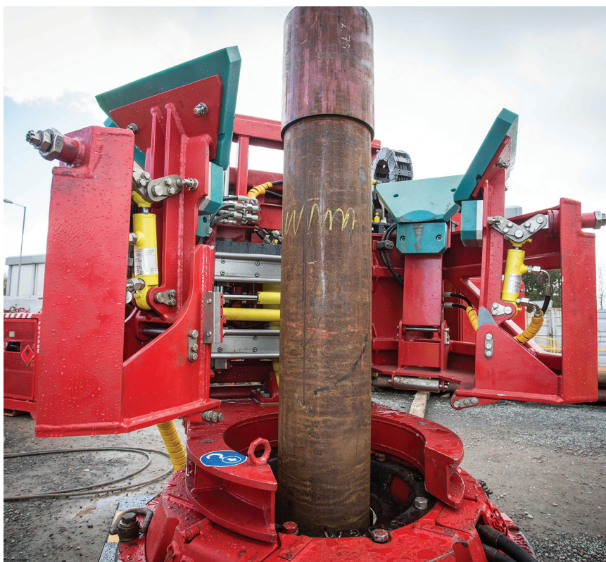
Fig. 1—Weatherford's mechanized stabbing guide enables automated stab-in of tubulars, which removes personnel from high-risk zones on the rig floor.
