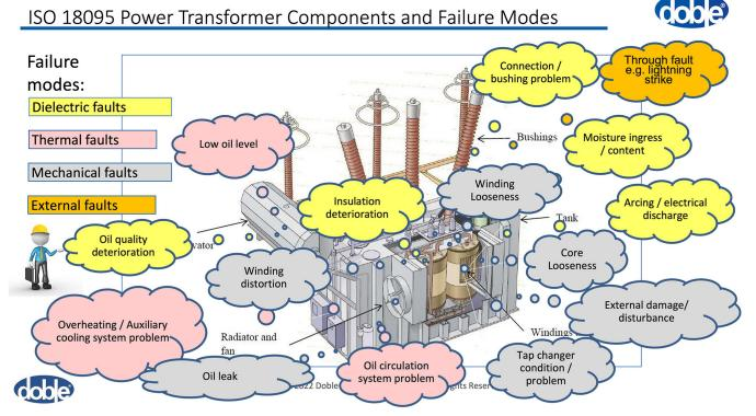
Figure 2. There are many potential modes of transformer failure per ISO 18095 [5]
