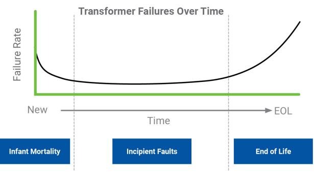
Figure 3. Transformer failure over time
