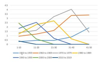
*Figure 4*. The failure rate of power transformers. Each line represents the failure rate of transformers produced in a particular decade
