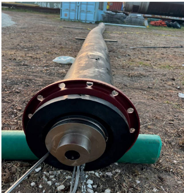
Figure 2. A hydrogen sensor, the HY-OPTIMA® 5031 from H2scan, is located in the annulus between the inner and outer carrier pipes. If the sensor detects that unsafe levels of hydrogen gas have leaked into this space, then a control system automatically initiates a purge of the annulus with an inert gas.
