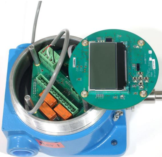
3. Plug the connector into the receptacle.
