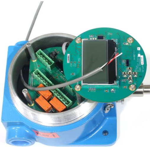
1. Insert wires through the conduit connections.
