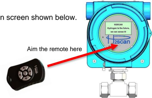
The screen will now display the Information Menu. Use the left and right buttons on the remote to scroll between menus. Use the up and down buttons as well as the middle button on the remote control to select and change settings within a menu.
