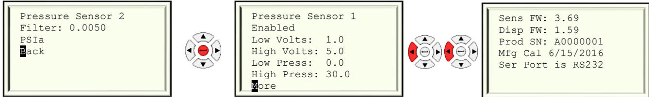
9. Exit the Information Menu by pressing the middle button on the remote control. The main screen will now have the pressure reading in atmospheres (atm), and the reported %H2 value is now pressure compensated.
