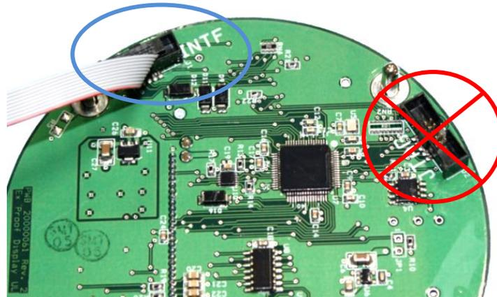
**Figure 2: Display Connections**
