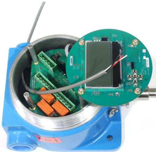
**1. Insert wires through the conduit connections.**
