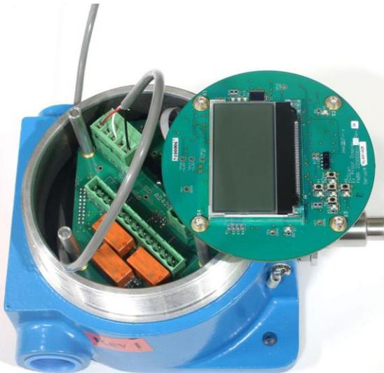
**3. Plug the connector into the receptacle.**
