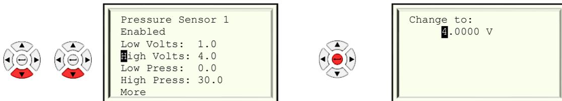
Use the left and right arrows on the remote to select the digit, the up and down arrows to change the value, and the middle button to save the final value.
