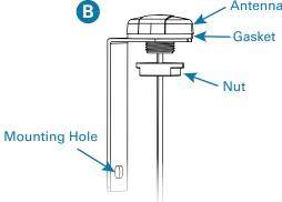
2B. Secure remote antenna bracket to a suitable location. Mount the antenna to the bracket by tightening the mounting nut to 3.9 Nm. Route cable to Sentinel Pro IOT Monitor (secure using cable ties as necessary) and connect, hand tighten only.
