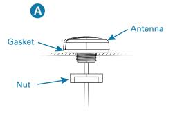
2A. Drill a 20mm (1") hole in the top of the enclosure. Feed the cable through the hole and the mounting nut.
