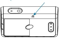
After 60 minutes all LED lights on the device will enter sleep mode. To reactivate the LEDs, place a magnet (activation tool) next to the magnet indicator (identified above) for 5 seconds.
