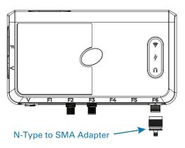
1. Attach the N-Type to SMA adapter to the Sentinel Pro Antenna port. Hand tighten only. Once antenna is mounted, route cable to Sentinel Pro IOT Monitor, securing with cable ties as necessary. Connect to Sentinel Pro IOT Monitor, hand tighten only.
