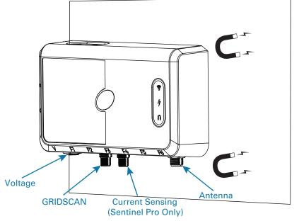
1. Attach Sentinel to a metal surface using built-in magnets. Ensure sufficient space under unit to attach cables.
