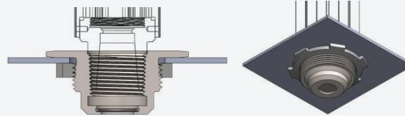
These mounting options ensure the HY-ALERTA 5020 sensor can be easily integrated into various environments, whether in rooms, enclosures, or outdoor settings, facilitating straightforward deployment setup.
