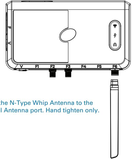
1. Attach the N-Type Whip Antenna to the Sentinel Antenna port. Hand tighten only.
