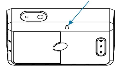
After 60 minutes all LED lights on the device will enter sleep mode. To reactivate the LEDs, place a magnet (activation tool) next to the magnet indicator (identified above) for 5 seconds.
