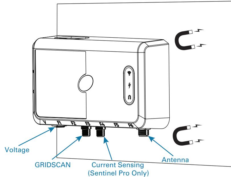
1. Attach Sentinel to a metal surface using built-in magnets. Ensure sufficient space under unit to attach cables.
