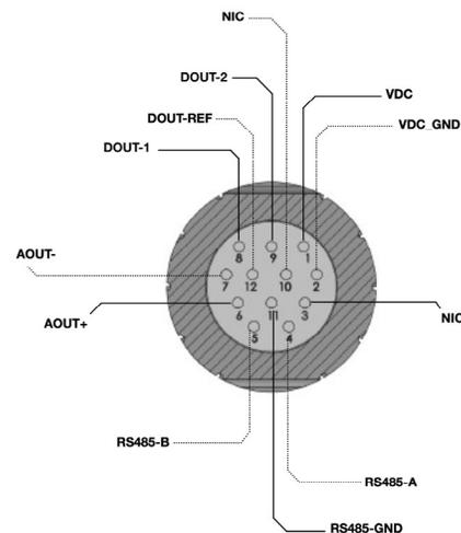
**Figure 3: H2scan Cable Pinout and Wire Colors**
