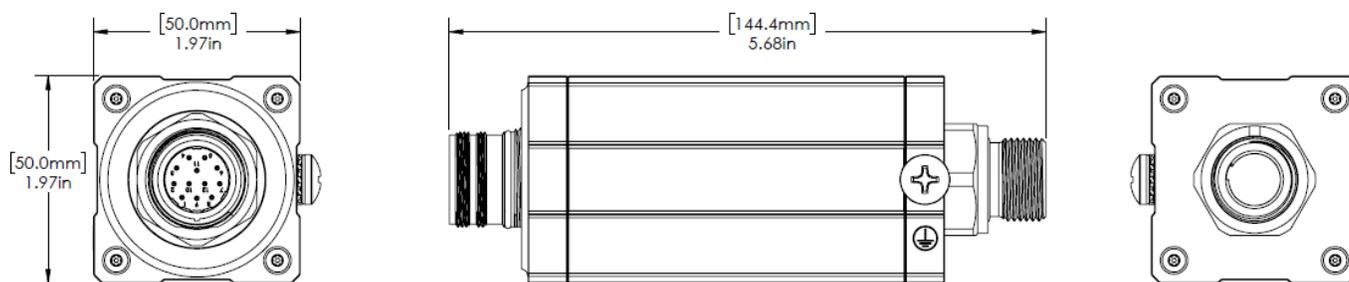
**Figure 1: HY-OPTIMA 5330 Series Hydrogen Analyzer Dimensions**
