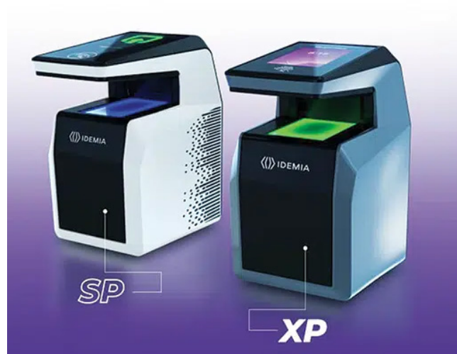
IDEMIA's MorphoWave contactless fingerprint solution scans and verifies four fingerprints in less than one second, through a fully touchless hand wave gesture, the company says. Idemia image.
