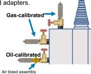
Apply liquid thread sealant or Teflon® tape on these locations
